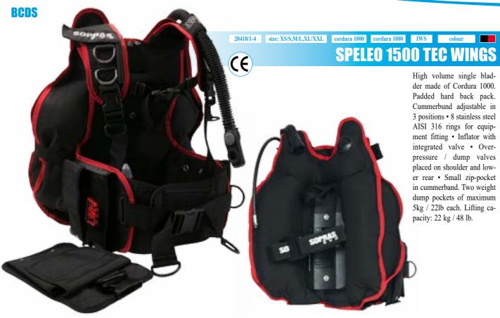
High volume single bladder made of Cordura 1000. Padded hard back pack. Cummerbund adjustable in 3 positions • 8 stainless steel AISI 316 rings for equipment fitting • Inflator with integrated valve • Overpressure / dump valves placed on shoulder and lower rear • Small zip-pocket in cummerband. Two weight dump pockets of maximum 5kg / 22lb each. Lifting capacity: 22 kg / 48 lb.
