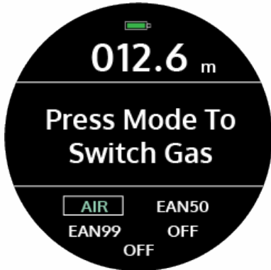
Tec Mode - Gas Switch (Before switching)
