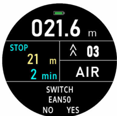
Tec Mode - Underwater Recommended Gas Switch
